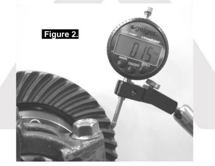
Set a depth indicator on one of the ring gear teeth as in Fig.2.
