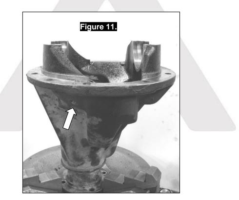
NOTE : It is a good idea to place a magnet on the inside of the differential housing to collect metal filings when drilling & tapping.
