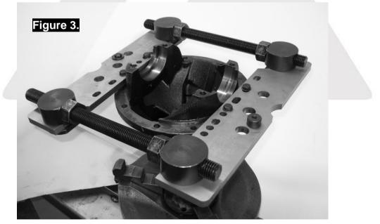
Release all spreader tension immediately after removing the differential carrier.
